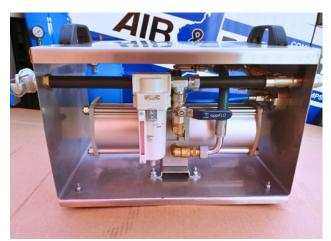
Tailored air multiplier designed for a client in the tyre industry. This innovation enables the client to double the pressure generated by their air compressor, enhancing tire inflation efficiency. Designed and manufactured in our Belmont workshop
