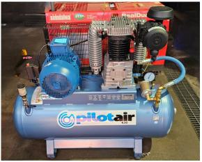
New PilotAir K30 was modified to include continuous running, allowing the compressor to run continuously without the need to start and stop. This reduces the strain on the generator greatly while in use. **Arc Infrastructure, WA**
